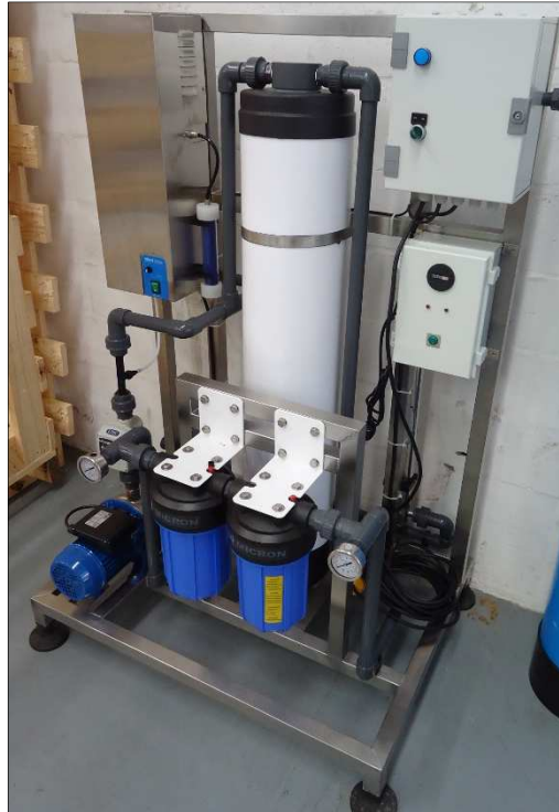
Figure 4: IL9 Filtration & Sterilization skid
