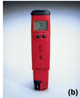
Fig. 2. (a) Laboratory quality pH meter and electrode with multiple reagents. (b) pH "pocket pal" for field monitoring of pH. (c) Volunteer uses a color comparator to assess pH (photo from EPA).
